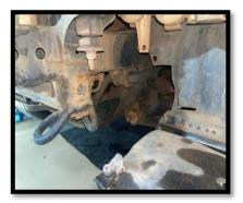
• Lightly tighten the winch plate and stiffeners supplied to the side and the front of the chassis.
